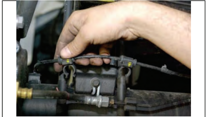
Vehicles with ABS/TC remove clips from U-bolts.
