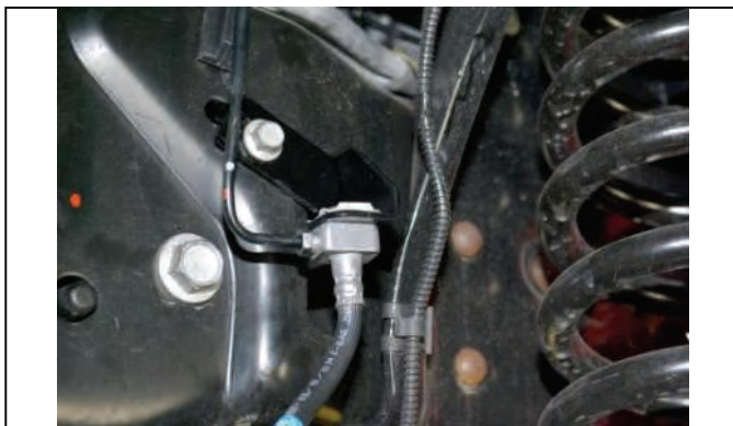
Reinstall block into bracket with retaining clip.
