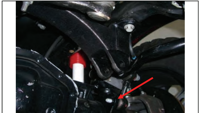
(05-10) Re-attach and tighten sway bar end links.
