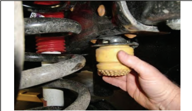
Remove bump stop and unbolt bracket from frame.
