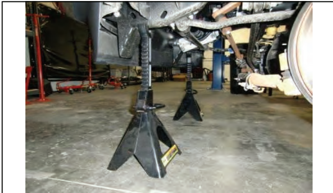
Lift front of vehicle and support with min. 3 ton jack stands.
