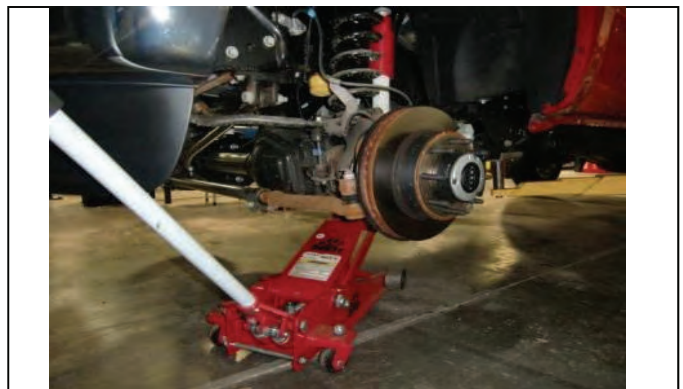
Support front axle with floor jack(s).
