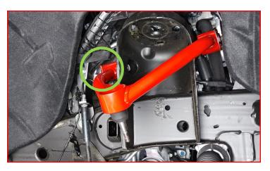
With the upper control arm bolts in place, install the supplied laser cut washers, the factory nuts and a drop of thread locker.
