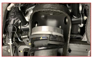
Install the factory lower strut bolts.
