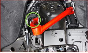
With the upper control arm bolts in place, install the supplied laser cut washers, the supplied M14 washers and nuts.
