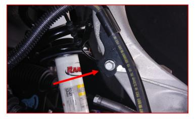
Remove the ABS bracket from the Upper Control Arm.
