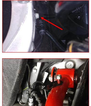
Install the ABS bracket to the Upper Control Arm using supplied 1/4" nut and washer.
