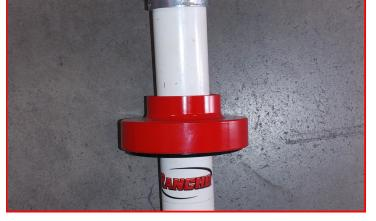
Install factory strut hardware on top hat studs. Mark studs at top of nuts.
