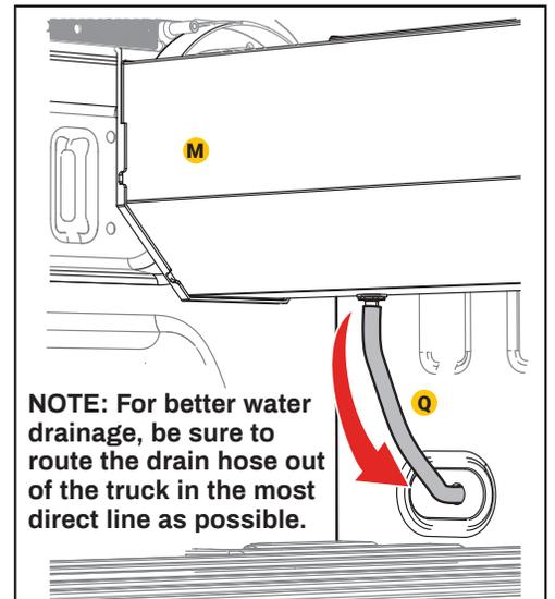
**NOTE:** For better water drainage, be sure to route the drain hose out of the truck in the most direct line as possible.
