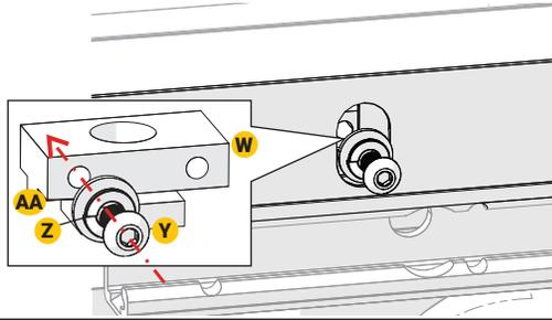
Before tightening the hardware, make sure the top of the RamBox rail is level with the top of the plastic bed rail cap. Do this on the driver and passenger side.
