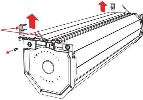
**11 Install the rails to the canister:** Pull the cover out of the canister (M) 6 to 8 inches, holding it from rolling back in, guide the cover into the rail (K & L) channel while positioning the rails into the canister (M). Align the front and rear rail attachment tabs and holes to the inside of the corresponding canister holes. **K**
