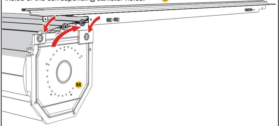
**12 Fasten the rails to the canister:** With the rails in place and the cover slid into the rail channel, attach the rails with the four 10-32 x 7/16" canister mounting screws (N).
