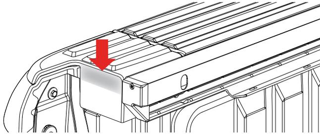
**5b.** Apply seal (GG) as shown below. Align seal flush along the top edge of the bed cap and the inner edge as shown. Apply pressure evenly to the entire seal to ensure proper adhesion. Do this on the driver and passenger side.
