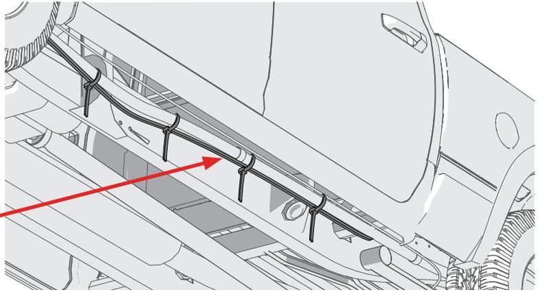
**7** Route the wire harness (D) to the driver side of the truck if it is not already. **Note: Using wire ties (E), secure the wiring harness (D) so it does not come into contact with moving parts or exhaust pipes.**
