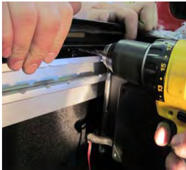
Hold drill level
