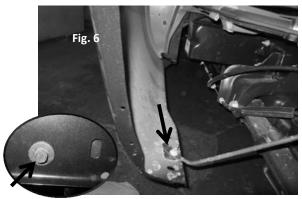
**8.** Insert one of the Medium size Push Pins into the pre-drilled hole attaching the liner to the truck frame (See fig. 7)
