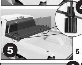
**4**. Secure cab clamp hooks under the metal bed rail. Toyota Models Only - Tighten lock nut at bottom of knob.
