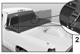
2. Undo both tie-down straps so cover can be unfolded.
