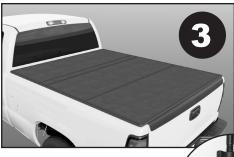
**3**. Unfold the cover all the way open to align cover on the truck bed rails before clamping.
