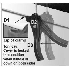
${f 8b}$ . To clamp cover down, put lip of clamp hooks under the side metal bed rail and push handle down. (See D1, D2, D3)
