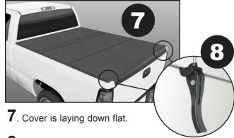
**8a**. Secure tailgate clamp hooks for a snug fit.
