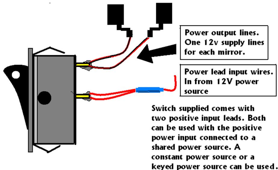
5. Connect the two 12V output lines (black-red) wires to the red power leads at each mirrors base. Each mirror will need one power supply line. Extra wire has been supplied for any additional wiring needs.
