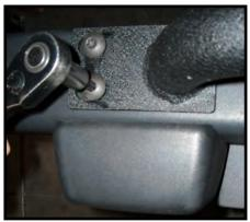
3. To use factory tow hooks with this light bar, place tow hooks on top of Light Bar mounting plates. Be sure to use the correct tow hook for each side of the vehicle. Tighten Light Bar into place using factory torx head bolts.
