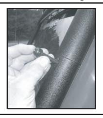
Step 9. Reinstall (2) torx head bolts to front of lower mounting bracket. With all (6) torx head bolts installed tighten securely to windshield frame. Tighten bolts in a clockwise rotation. Tighten M8 Allen head tube bolt. Repeat for other side.
