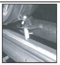
Step 7. With lights mounted install top light bar with the help of a second person. Attach wire connectors and place onto lower mounting tubes. Lower mounting brackets may need to be pulled outward to allow top tube bar to slide into position.
