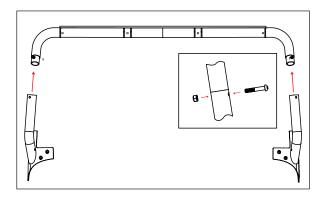
3. Remove the factory left and right windshield brackets. Retain factory hardware for later use.
