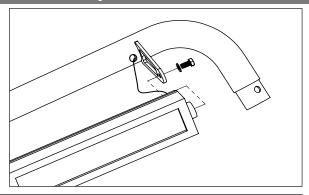
2. Attach left and right brackets to front crossbar with supplied M10x60 bolt and nylon lock nut. Do not tighten completely to allow for adjustment.
