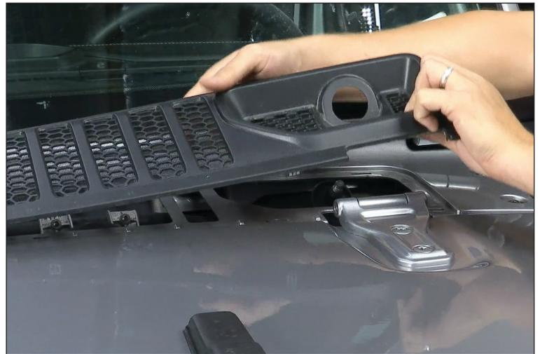
3. Next install the hood hinge mount. Begin by removing the OE 13mm bolts from the hood hinge. You'll notice the bolt location is staggered. The lower bolt is on the outside. Make sure the hood hinge staggered holes aligns with the hinge holes. Reinstall the OE bolts and tighten.
