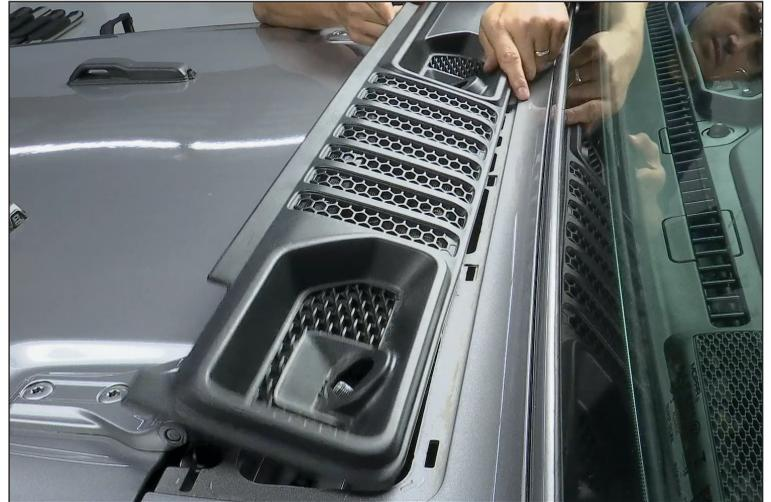
5. Attach the light bar mount. Depending on the size of the light bar you are mounting the mounts could point in or out. Place mount in front of the Hood hinge mount and tighten using the black Teflon coated M8 hardware provided.
