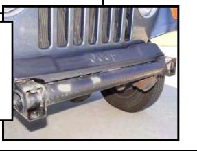
**Step 2:** Position the new bumper up to the frame and line up the holes to the factory mounting locations. Using the included and factory hardware, secure the bumper to the vehicle and tighten the bolts.
