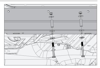
18. Attach Rock Slider Panels to 4 body mount tabs through 4 mounting slots using M6 Hex Bolts, M6 Large and Small Washers, and M6 Lock Nuts.
