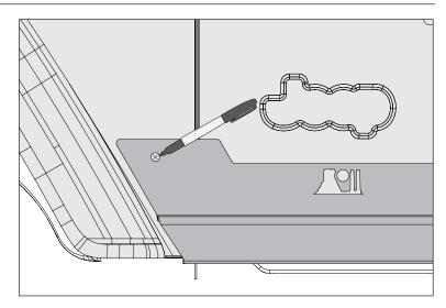
5. Beginning with a 3/16" bit, drill 6 mounting holes into side body. Continue with 7/16" bit for front 4 holes and 9/16" for rear 2 holes to finish full diameter of mounting points. Clean any metal chips and shavings from vehicle before continuing.
