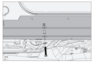
17. Attach remaining bottom holes using M10 Long Hex Head Bolt, Flat Washers, 45mm Spacer, and Lock Nuts.
