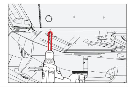
15. Attach side mounting holes in Rock Silder Panels using M10 Button Head Bolts, Flat Washers, Lock Washers, and M10 Nuts.
