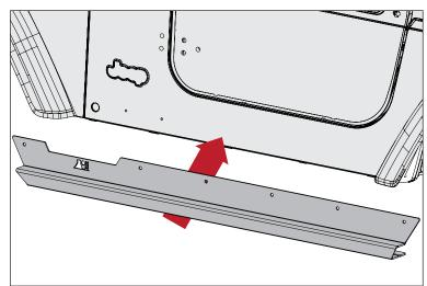
4. Once positioned, mark and center punch 6 side holes for drilling.
