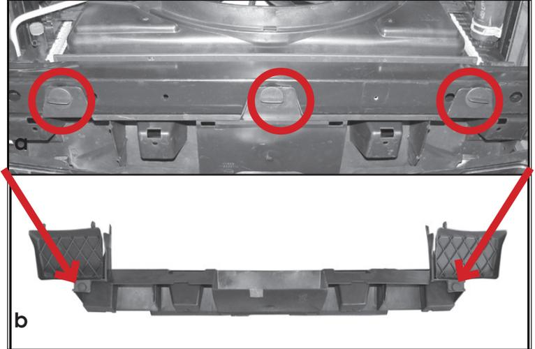
**2014 Models:** The block offs covering openings in bumper are clipped onto back of bumper cover only. Remove hardware at bottom of inner fender panel (a). Release clips behind bumper and remove block off from each opening in bumper cover (b).
