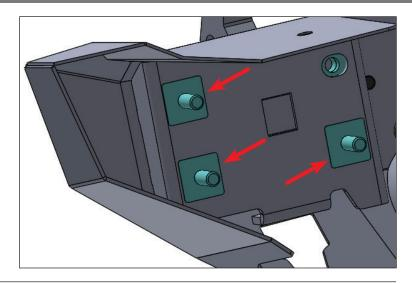
5. Now lift and place the bumper to the Jeep frame rails. The studs slide through the holes in the frame holes. It's best to have an assistant to lift and hold the bumper in place.
