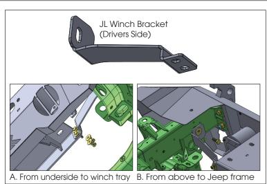
9. Now install passenger side JL winch bracket. The bracket mounts to the winch tray with two M8 bolts with flat, lock washers and nuts. Next mount to the Jeep frame with M10 bolt and flat washer.
