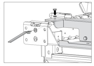
16. Position Bumper Assembly over frame rails, aligning Tow Hooks with mounting holes on frame horns. Secure with OE Nuts.
