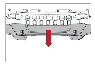
2. Disconnect turn signal from behind grille. Rotate bulb assembly down and pull out of light housing.
