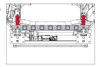
6. Unbolt and remove factory vacuum pump. Retain factory bolts.
