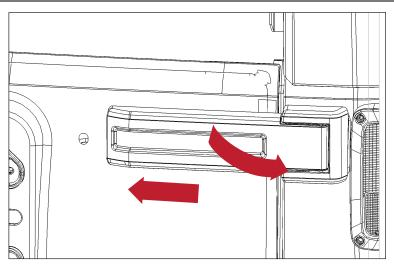
6. Remove plastic clips by pulling lower portion down and away from vehicle.
