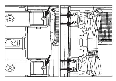
13. Re-using factory bolts and washers removed in step 6, loosely attach right side of HD Hinge Casting.
