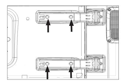
10. Flip hinges to open position. Using a T-50 bit, unscrew stock hinges from vehicle removing the screws indicated at right. This may require using a 10inch extension with the T-50 bit in order to reach the scews.
