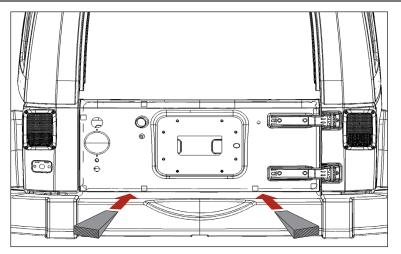
9. Using 13mm socket, remove tailgate hinges from tailgate by removing the 4 bolts indicated on right.
