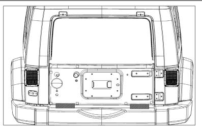
12. Place HD Hinge Casting in position. Reusing 6 factory screws, fasten hinge brackets to vehicle quarter panel. Attach outside screw first, then swing hinge open and install remaining four screws.
