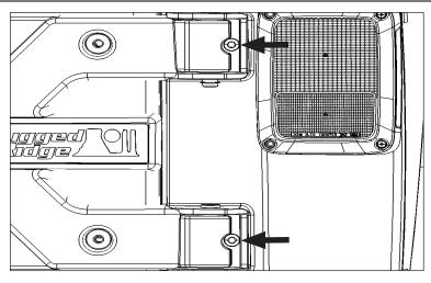
15. Remove the 4 bolts/washers from Step 12. Swing HD Hinge Casting open, making sure not to move the tailgate. Tighten the 4 remaining Torx Head bolts on hinge brackets. Return to closed position.
