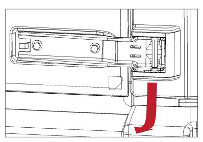
7. Remove the stock tire carrier and brake light holder by removing the 8 bolts indicated using a 13mm socket.
