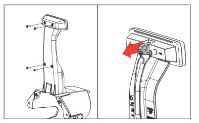
4. Twist and pull rubber bumper to remove from right side of tailgate only.
