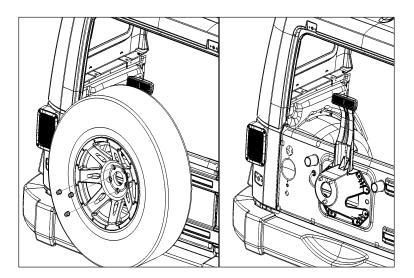
2. Open the tailgate. Using a T-20 Torx bit, remove 4 torx head screws that attach light to factory tire mount. Pull light away from tire mount.
