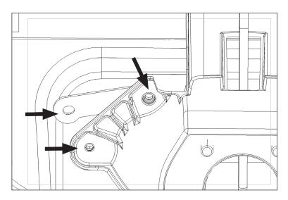
19. Once all bolts are threaded, tighten the 8 bolts around the tire carrier.
