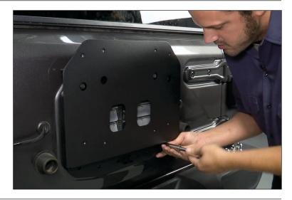
3. Using an assistant, install spare tire. Tighten lug nuts to 80ft lbs torque.
