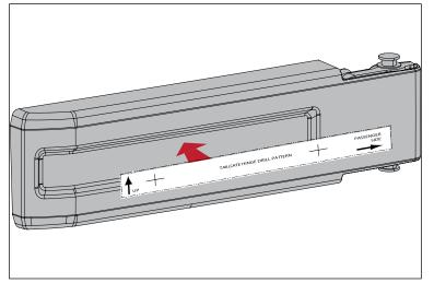
3. Remove upper left tailgate hinge bolt. Use M8 hardware and spacer to secure Upper Mounting Plate to left hole of upper tailgate hinge. Do not fully tighten.
