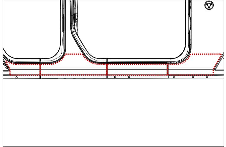
2. Using painter's tape, place driver side cladding pieces on vehicle. Align with vehicle door opening and fenders.
