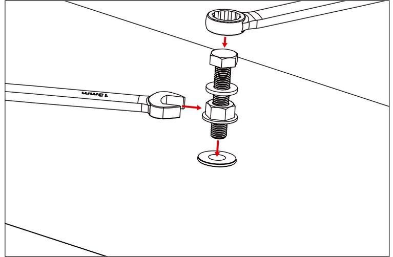
6. Mount Front Cladding using collapsed Rivet Nut and supplied M10 hardware.
