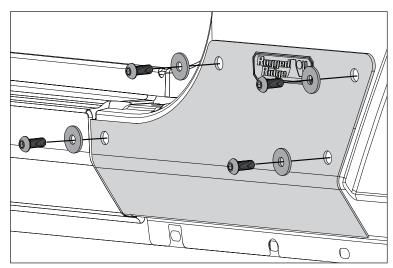
7. Repeat steps 3-6 for remaining cladding pieces on driver side while working from front to back of vehicle.
