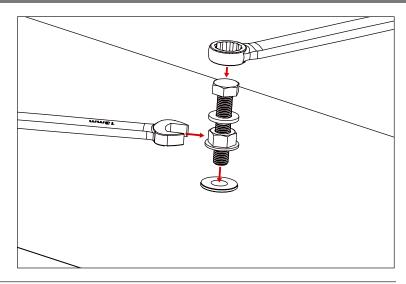
6. Mount Front Cladding using colapsed Rivet Nut and supplied M8 hardware.
