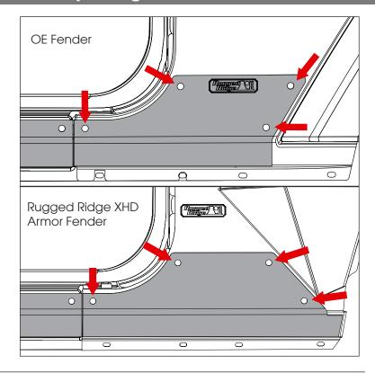
4. Using 1/8" drill, make a pilot hole at four marked locations. Using a step bit, open hole to 13.5mm. For some locations the Cowl Side Panel behind the fender will also need to be drilled out too allow fitment of Rivet Nut.
