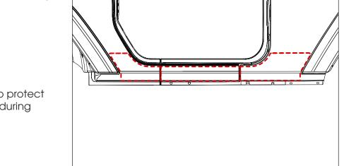
Painter's tape can be used to protect vehicle paint from scratches during installation.
