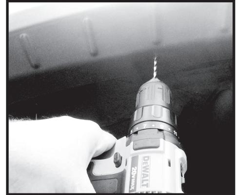
Step 26. Secure the flare to the wheel well using the supplied #8 screws. Do not over tighten screws.
