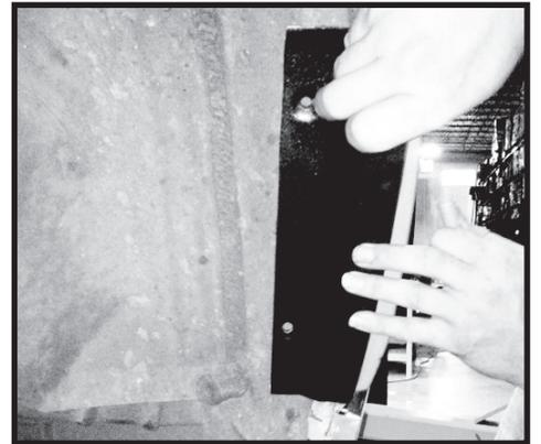
Step 39. Hold the flare against the body using slight pressure to check fitment. Some trimming and sanding may be necessary to flare may be needed to ensure a smooth fit to the body. Once the correct fit is achieved trace a line onto the lower body cladding of the rear door. This area of the cladding will be cut to match the curve of the flare.
