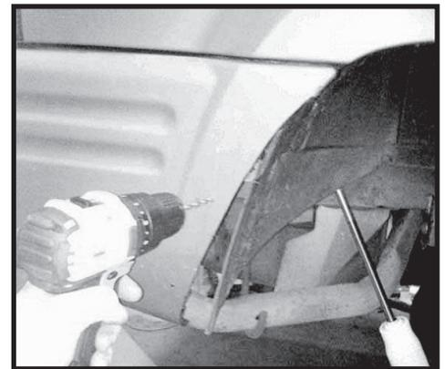
Step 59. Attach the L shaped brackets to the rear bumper cover as shown. The brackets will mount to the inside of the bumper cover and using a bolt and nut with a washer on each side of the bumper cover.
