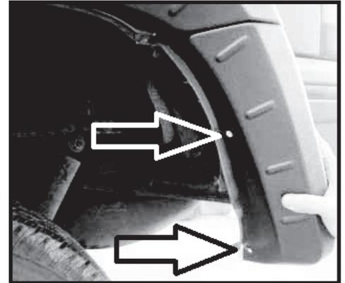
Step 58. Drill two mounting holes into the rear bumper cover using a 3/16" drill bit.
