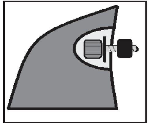
Step 23. Position flare against the body over the drilled mounting holes. Start each screw into the mounting holes. Once each screw has been started, snug the flare to the body. **DO NOT TIGHTEN.**
