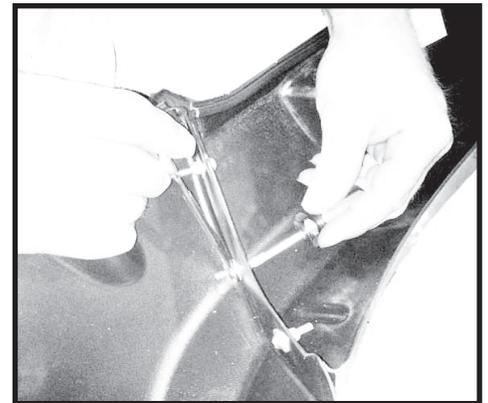
Step 51. Hold assembled flare sections in place on the vehicle. Due to the multiple body cladding styles the flares may not have a completely flush fit. Some sanding and contouring may achieve desired results. Use caution when modifying flares. Do not remove material from around bolt hole mounting areas.
