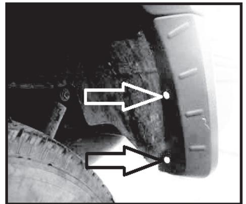
Step 63. Using a 3/32" drill bit, make pilot holes into the fender well using the pre-drilled holes in the fender flare as a guide.
