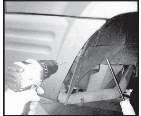
Step 62. Reinstall the rear bumper cover splash shield using the factory hardware previously removed. Attach the lower rear portion of the fender flare to the two L brackets on the rear bumper cover using two plastic push rivets.
