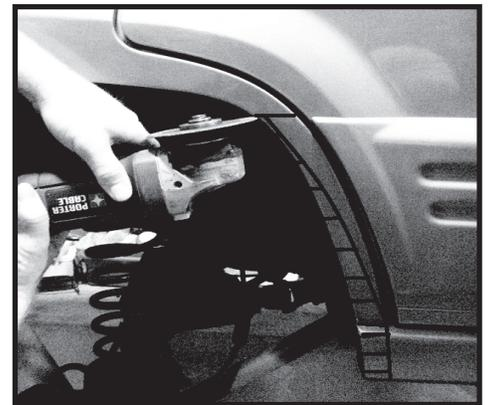
Step 35. Using pliers bend the cut fender well lip out. Bend only one section at a time. Bend the lip out so that it creates a flat, even surface, flush with the outside of the fender.
