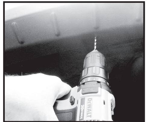
Step 64. Secure the flare to the wheel well using the supplied #8 screws. Do not over tighten screws.
