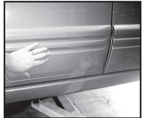
Step 48. Install the lower rear rocker panel end cover. Mark the mounting holes for the lower rear rocker panel end cover. The cover is held on with two self tapping screws on top and bottom of the cover and one body mounting bolt on the front.
