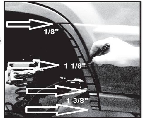
Step 34. Using a cutoff wheel or sawzall cut the lines made on the fender. Cut only the horizontal lines from inside of the fender to the vertical line drawn. Use caution when cutting. Do not over cut or cut into surrounding areas.
