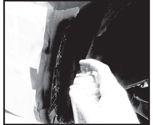
Step 38. Hold the door jam cover supplied in place over the front section of the wheel well behind the rear door. Panel should cover area previously modified. If the door jam cover does not fit smooth and line up with the door jam then more bending modification will be needed to wheel well. With cover in place mark the two mounting holes. Remove cover and drill marked areas with a 3/32" drill bit. Attach panel using the supplied phillips head screws.
