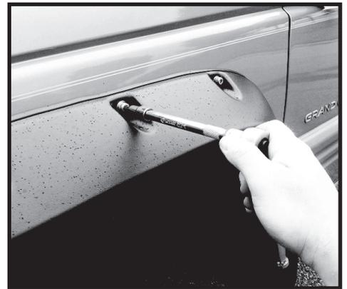
Step 24. Torque each bolt to 24 in-lbs (2 ft-lbs). Do not over tighten. Over tightening could cause damage or warpage.
