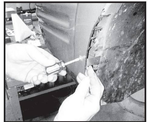
Step 60. Hold the flare against the body using slight pressure to check fitment. Some trimming and sanding may be necessary to ensure a smooth fit to the body. Once the correct fit is achieved mark the mounting holes on to the body using the holes in the flare as a guide.
