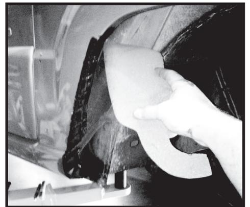
Step 7. Remove the lower fender bolt located at the bottom rear of the front fender. Measure 2 inches back from the hole towards the rear of the vehicle. Drill a 3/16" pilot hole. Reinstall the bolt removed previously.
