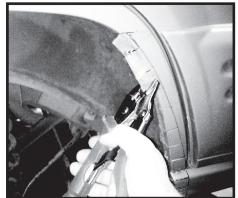
Step 36. Using a heavy hammer bend the tabs inward. The tabs should start at the line drawn and should be bent inward 90 degrees towards the fender well duplicating the factory bend.
