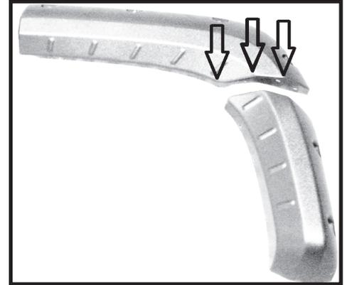
Step 50. Attach the rear and middle wheel arch flare sections using the supplied bolts and lock nuts with a washer on each side of the flare flange.
