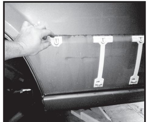
Step 45. Hold the flare against the body using slight pressure to check fitment. Some trimming and sanding to the flare may be necessary to ensure a smooth fit to the body. Once the correct fit is achieved mark the mounting holes on to the body using the holes in the flare as a guide.
