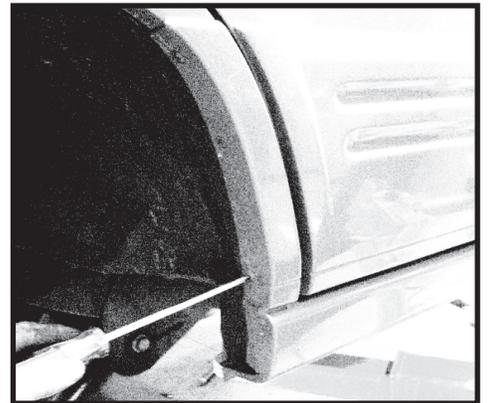
Step 32. If your vehicle is equipped with a plastic rocker panel cover, you will need to draw a vertical cut line and trim the cover. The line will need to start from the bottom point of the door trim and extend downward. A razor knife will be suitable for trimming. Ensure the cut is smooth, this area will be visible after the flare is installed. After trimming, the panel cover should be slid forward slightly or removed when cutting the body.
