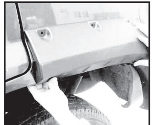
Step 53. With the flare in place trace the edge of the flare onto the rear bumper. This area of the bumper will be trimmed for proper fitment of the flares.
