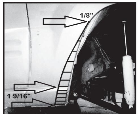
Step 9. Using a cutoff wheel or sawzall cut the lines made on the fender. Cut only the horizontal lines from inside of the fender to the vertical line drawn. Use caution when cutting. Do not over cut or cut into surrounding areas.
