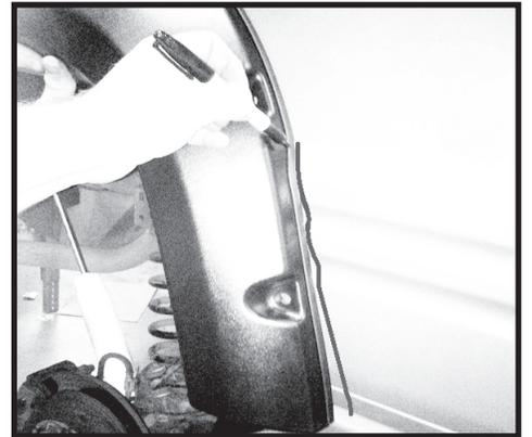
Step 40. Remove the retainer nut from the backside of the rear door that holds the lower body cladding on to the vehicle.
