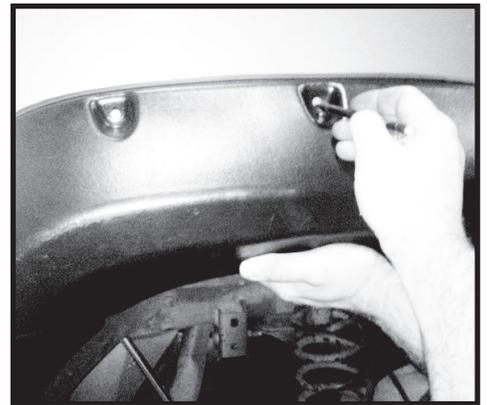
Step 20. Drill holes marked on fender using a 3/16" drill bit.
