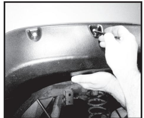
Step 61. Drill holes marked on fender using a 3/16" drill bit.
