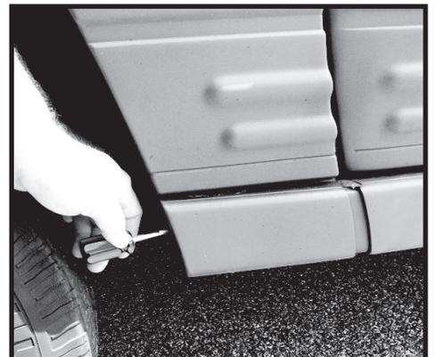
Step 5. Remove the front wheel well liner. Liner is held in by plastic fasteners. Use caution as not to damage fasteners when removing. The fasteners will be reused later to reinstall the liner.
