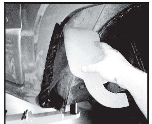
Step 17. Reinstall the inner fender liner. Some of the mounting holes have been removed with trimming of the wheel well. New mounting holes can be made or use zip ties to hold the liner in place.
