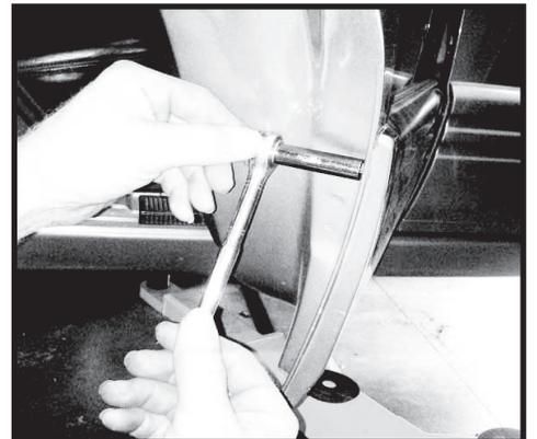
Step 41. Remove the body cladding from the vehicle. First, lift up the top edge to release the upper portion of the cladding. Next pull bottom of cladding straight out from side of vehicle.
