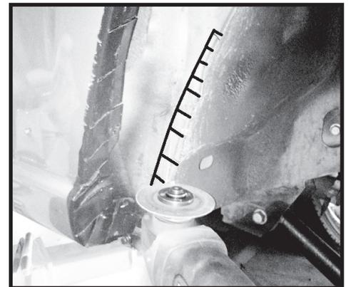
Step 15. Bend the cut tabs inward towards the fender well. Using a hammer bend them as close as possible to the fender well. Flatten all sharp areas. Remove all loose paint chips and sand rough areas. Mask off area and coat with a rust inhibiting paint.
