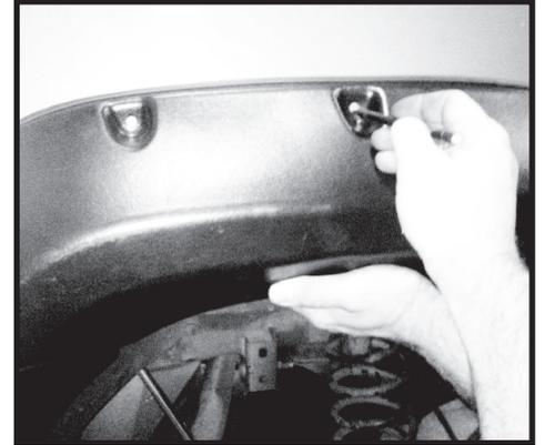
Step 46. Drill holes marked on fender using a 3/16" drill bit.
