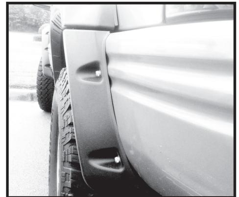
Step 52. Hold the assembled rear sections of flares against the body aligning the front area of the flare to the body crease behind the rear door opening. Adjust the flare to achieve a 1/4" gap between the wheel arch flare and the door flare.
