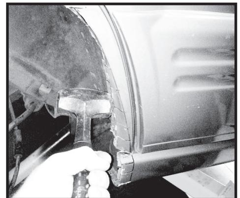
Step 37. Remove all loose paint chips and sand rough areas. Mask off area and coat with a rust inhibiting paint.
