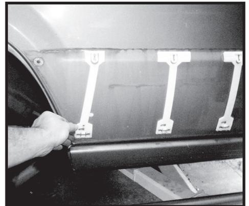
Step 44. Trim the retainer just below the upper clip portion and reinstall onto the door.
