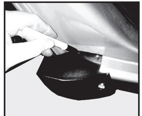
Step 49. Assemble the rear and middle wheel arch flares. Align the two rear flare sections by the three style line areas indicated. Once the pieces are aligned mark the holes on the inside mating lip from one flare to the other flare. Drill holes with a 1/4" drill bit.
