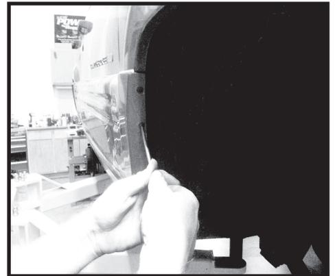
Step 3. Once screws have been removed cladding will snap off from vehicle. Remove cladding and retainer from vehicle. Discard cladding and retainer. There are two mounting pins on the fender. These may need to be trimmed from vehicle to ensure proper fitment. Treat any unpainted surfaces to prevent rust.
