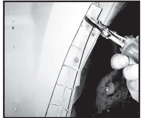
Step 11. Bend the tabs inward. The tabs should start at the line drawn and should be bent inward 90 degrees towards the fender well duplicating the factory bend.
