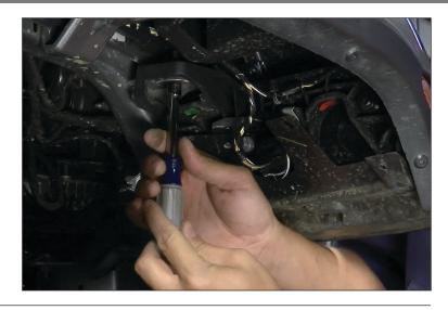
5. Pull splash shield down to reveal additional T25 torx screws to remove.
