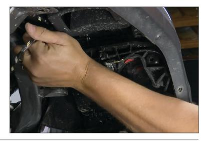
8. Now release all the white retaining clips that attach the fender to the Jeep. Use a small set of needlenose pliers to pinch the back side of the clip and pull the fender from the Jeep. The last clip at the bottom of the fender is deep in the fender. Standard needlenose pliers won't reach it. You could use a long screwdriver or just pull to release this clip. Now fender can be removed.
