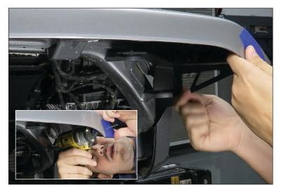
15. We choose to use a step bit to fit the desirable size. You can use standard bits if you prefer. Drill and build up to the size hole needed for the LED light. Test fit the light to assure it fit's snug.
