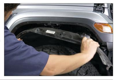
2. Remove the lower fender brace located at the rear bottom of the fender.
