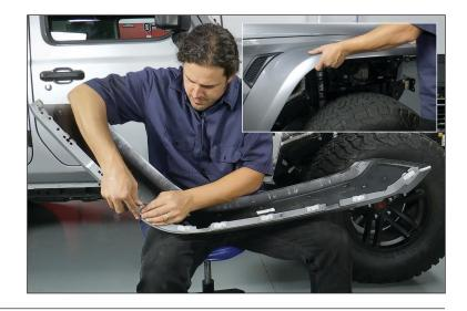
14. Next you need to mark and drill the hole for the side marker light. First apply painters tape to the fender to assist in keeping the paint from being scratched. Now loosely install the Chop Bracket with the 2 fender mounting bolts. Mark the inside of the fender in the center of the hole of the fender bracket. Remove the bracket and drill a pilot hole to the mark you made.
