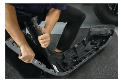
12. The locating tabs need to be trimmed away. A shape box blade works well cutting through the plastic. Feel free to use other tools if you feel fit. Take your time don't rush or force your cut. That could accidently cause you to cut to far or scratch the paint.
