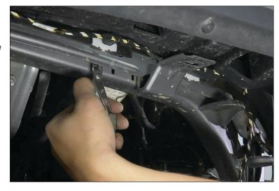
9. Place the fender on a soft surface to assure the paint won't be scratch during modification. First pry and remove all the fender clips to reuse later. Also remove wiring harness from fender.
