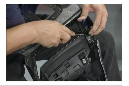
11. Remember to place fender on a soft surface. Now pull the inner fender away from the out fender. These items are glued or fused to each other. Start at the bottom corner of the fender and pry the pieces apart from each other.
