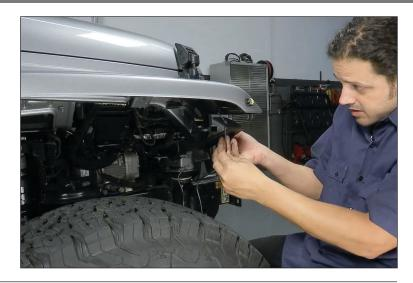
17. Use the provided M6 bolts and washers and attach the bracket to the fender tabs. Adjust and fully tighten.
