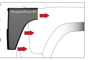
9. Firmly hold the Body Armors in proper mounting position while pulling the exposedplasticlinertocompletelyremove. Maintain pressure on installed itemfor30secondstoensurepropercontact.Fulladhesionoccurswithin24 hours of application.
