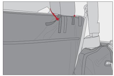
11. For more coverage, attach flaps on sides of seats, folded and secured in step 8, to hook and loops strips near rollcage.
