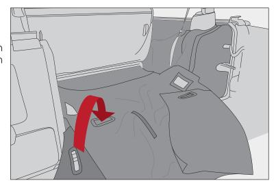
9. Ensure all footman cut outs are aligned and open and fabric is pushed into crease at base of seat. Lower seats to riding position.
