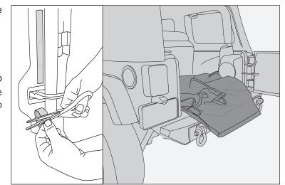
5. Attach hook and loop strips around base of rollbar and seatbelt.
