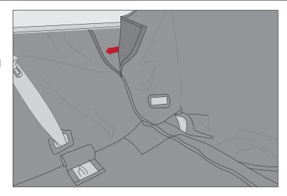
16. Secure bottom corner flaps to corresponding hook and loop strips.
