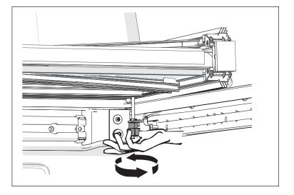
Close the tailgate and unfold the cover. Check that the cover is parallel and square with the truck bed and bed rails. If not parallel or square, open the cover and loosen the cab clamps to reposition the cover.
