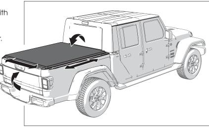
9. NOTE: When opening the cover, be sure to stow the tail clamps into the cover bow to prevent damage to the tarp when folded.
