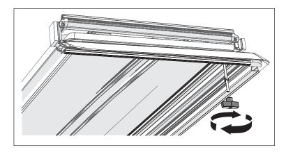
6. Place the cover onto the truck bulkhead and bed rails, making sure to slide the cab clamp threaded rods (2) through the cab clamp brackets (3). Align both sides.
