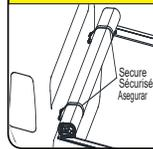
Before driving with cover open, BOTH STRAPS MUST BE SECURED TO RETAINING LOOPS. Failure to do so could cause accidental release of the cover, resulting in personal injury or property damage.
