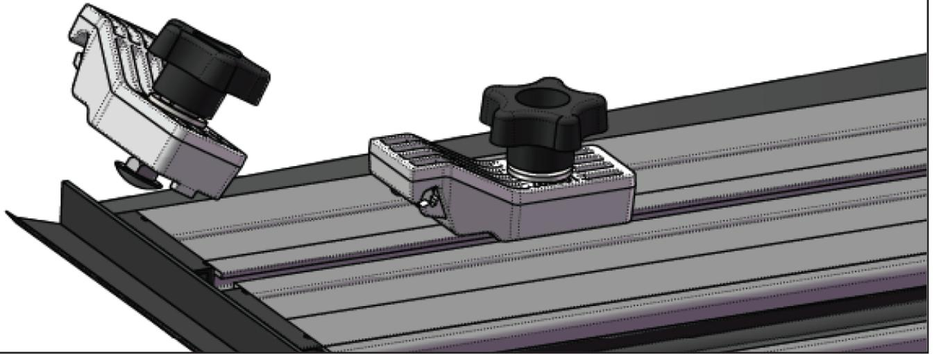
6 & 7. Slide the two front pre-staked cover retainer assemblies into the track on the underside of the tonneau cover, do not remove bolt from assembly.
