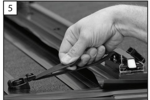
3, 4 & 5. If this is as far as you would like to open the cover, you can secure it in this position. Release the strap from the stowed position by squeezing the tabs. Attach the buckle at the bulkhead, pull the strap to take up the slack and secure the cover. Repeat this for the opposite side.
