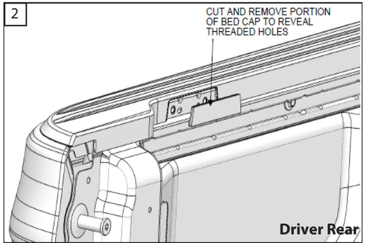
2. Locate the outlined section on the inside of the bed cap towards the tail light well at the rear of the bed. Cut and remove the outlined section of bed cap to reveal threaded holes. Repeat process for both Driver and Passenger side.
