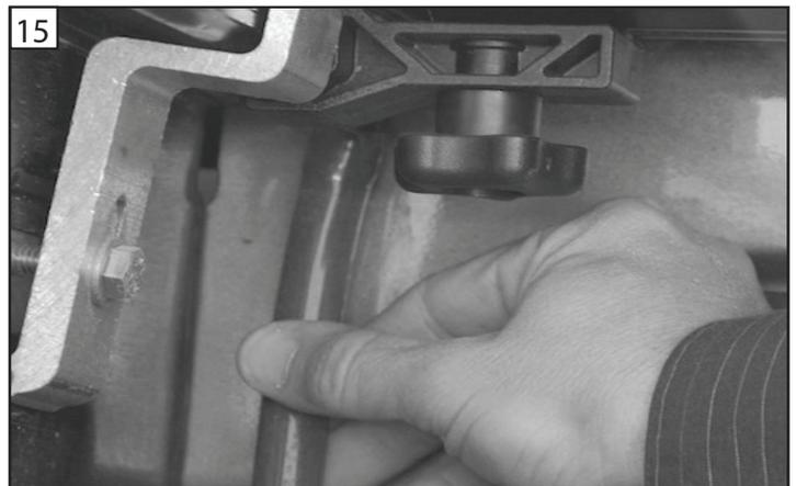
15. Attach the drain tubes to the fittings at the front of the bed rail and position the tubes to divert water out of the truck bed. This can be done by placing the tube behind a bed liner, through an existing hole in the bed, or by drilling a 5/8" hole in the bulkhead.
