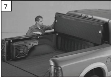
6 & 7. Pull the cable on the third panel and fold the cover up towards the cab.
