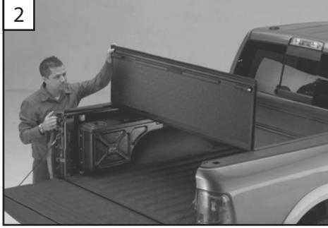
1 & 2. To open the cover: Lower the tailgate and pull the cable. While pulling on the cable lift the panel up and towards the cab, repeat for the next panel.
