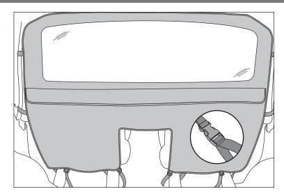
5. Zip windbreaker to tonneau cover using zipper under flap of windbreaker.
