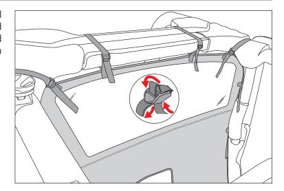
3. Thread side straps loosely around side sport bars as shown.
