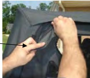
Start at the rear and roll the plastic along the bottom of the panel into the retainer on the vehicle. Then fasten the hook and loop strips along the rear of the panel to the top.
