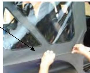
**Step (13):** Insert the tailgate bar into the mounts on each side of the tailgate opening with the vinyl side of the rear window towards the outside of the vehicle.
