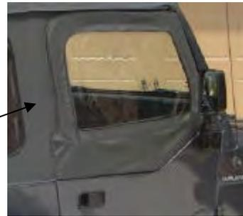
**Step (18):** Reinstall the upper doors. Insert the pins into the grommets in the lower door.
