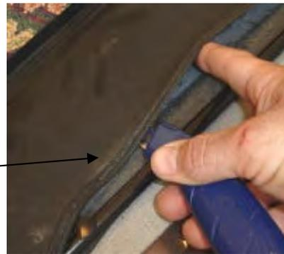
**Step (16):** Unzip the windows and separate the hook and loop fasteners on the door covers. Lay the door cover on a flat surface with the outside facing down. Start by working the lower rear corner of the door frame into the pocket in the lower rear corner of the cover. Then work the lower front corner of the frame into the cover. Work the top front corner of the frame into the corner of the cover, between the hook and loop flaps (not between the zipper and the flap).
