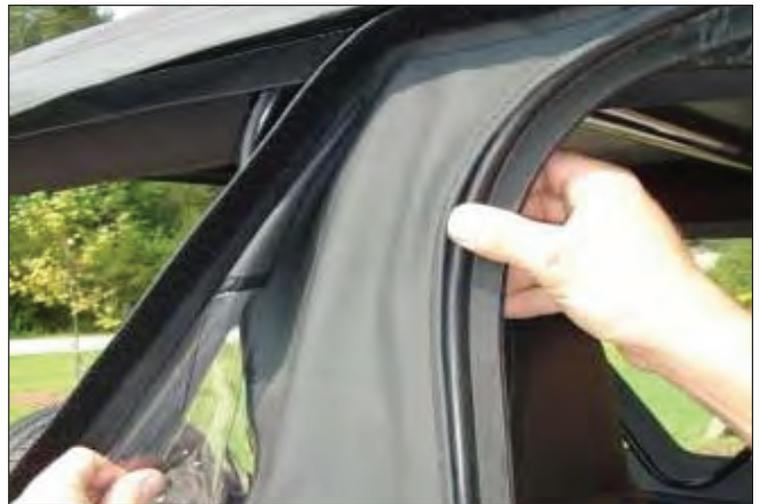
14. Locate plastic strips on each side of top and insert into door surrounds above door opening.
