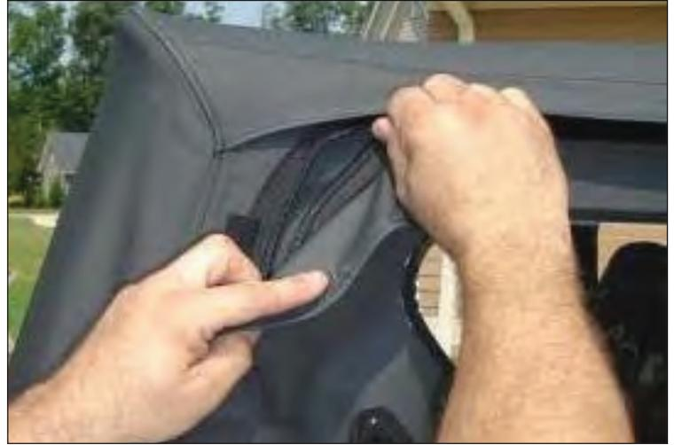
16. Start at rear of vehicle and roll plastic lip along belt rail. Fasten hook and loop strips that connect rear of side window to soft top.
