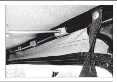
4. Remove screws that secure top to bow above roll bar and set aside for later use.
