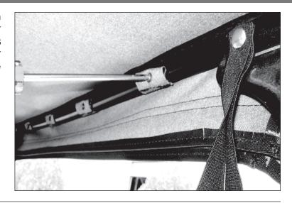
10. Reattach screws that secure top to bow above roll bar. Reattach cable spring to center bow using needle nose pliers and replace fabric spring cover.
