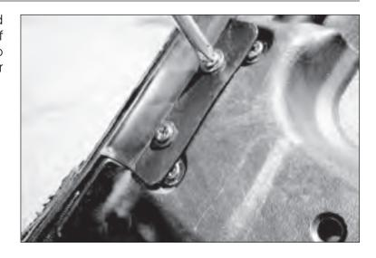
9. Raise top and bow assembly in upright position and lock header to windshield. With top loosely over bow assembly, reattach fabric to bows using screws removed in step 3. Fabric on rear bow wraps under bow from back to front of vehicle. Fabric on middle bow wraps over bow from front to back of vehicle.
