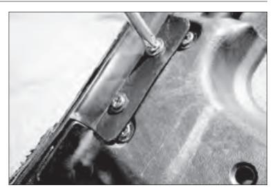
6. Raise top and bow assembly in upright position and lock header to windshield. Carefully drape soft top fabric over windshield and remove all screws from top side of header. Remove top of header and soft top fabric.
