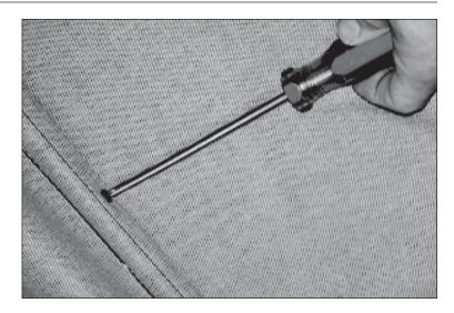
5. Lower soft top and remove screws that fasten soft top fabric to bottom corners of header. Set screws aside for later use.
