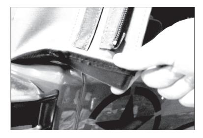
12. Insert tailgate bar into new rear window and install rear and side windows. Inspect top over door surround to ensure cable is tight.
