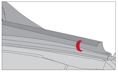
7. Locate ceiling adjustment straps at rear corners on ceiling panel. Gently pull strap over rollbar and around seatbelt stud and back up to strap adjustment buckle. Tighten snugly and repeat other side. Check top for evenness from side to side.
