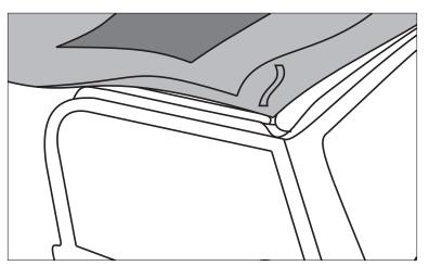
5. Insert front plastic into groove of Windshield Channel. Ends will match nearly to each end of Windshield Channel. From front of vehicle, ensure that top is even from side to side. Check door surround sides and push top toward rear to ensure fabric is seated tightly around front corners.
