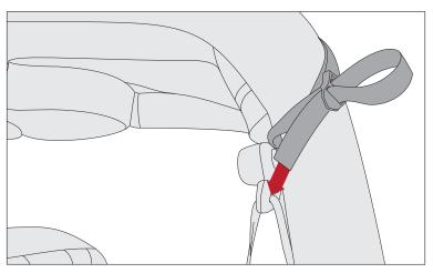
8. Install side windows by mating zippers. Loosely attach rear window to three straps on top rear. Mate rear window zippers to top on both sides and zip down about 6".
