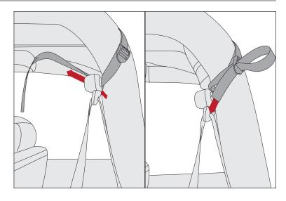
16. Install whisper bar by first inserting from front of vehicle over center sport bar.
