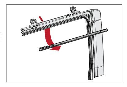
4. Attach bowless top to header by looping top over header channel and fastening with snaps on underside of header.
