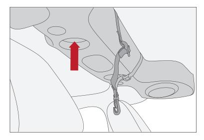
12. Pull two rear straps around rear sport bar and through plastic buckle. Tighten both sides.
