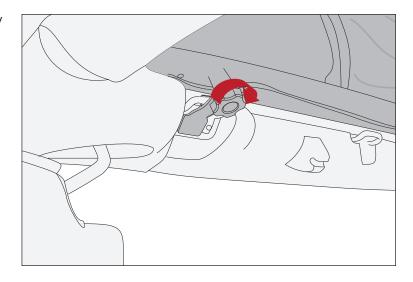
8. Hook side plastic retainer over front door surround and hook into groove over front door. Repeat in "X" pattern for front and rear door surrounds (front left, back right, front right, back left).
