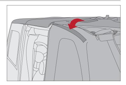
25. Insert remaining side window plastic retainers into groove of body tub. Repeat for opposide side.
