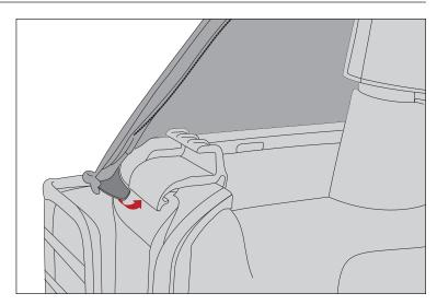
26. Slide tailgate bar into bottom of rear window and attach to receiver on tailgate.
