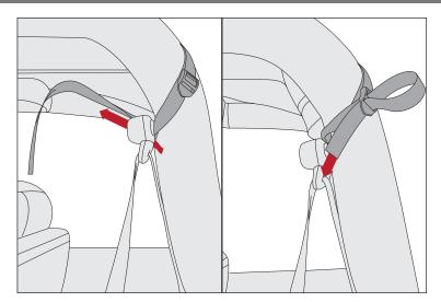
14. Install whisper bar by first inserting from front of vehicle over center sport bar.
