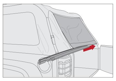
25. Install metal hook on end of rear straps into body tub through cutout in rear panel and tighten. Repeat for opposite side.
