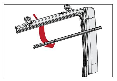
4. Attach bowless top to header by looping top over header channel and fastening with snaps on underside of header.
