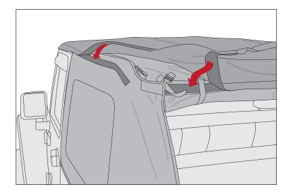
23. Insert remaining side window plastic retainers into groove of body tub. Repeat for opposide side.
