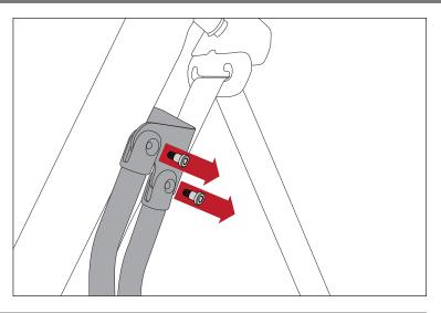
2. Remove metal soft top mounting brackets attached to roll bar in cargo area.
