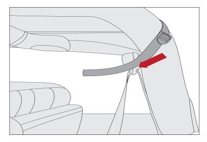
12. Loop strap under seatbelt stud, then back around to outside of vehicle.
