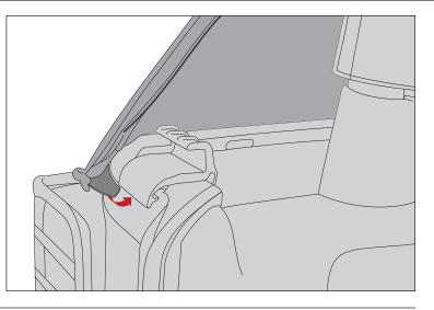
24. Slide tailgate bar into bottom of rear window and attach to receiver on tailgate.
