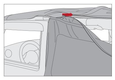
19. Pull bottom plastic retainer of side window into side groove of body tub. Repeat step 17 - 19 for opposite side.
