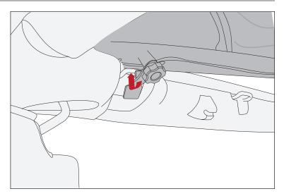
7. Ensure header is flush with windshield and screw plastic knob into header on each side of vehicle.
