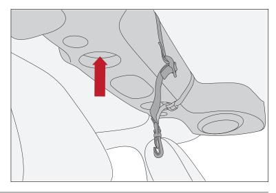
11. Loop rear side strap around rear sport bar, moving toward outside of vehicle.
