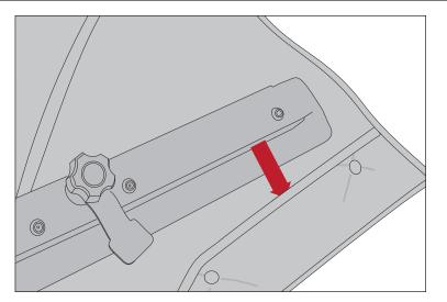
5. Slide bowless top to front of vehicle, placing it over sport bar.
