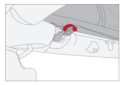
8. Hook side plastic retainer over door surround and hook into groove over front door. Repeat for opposite side.
