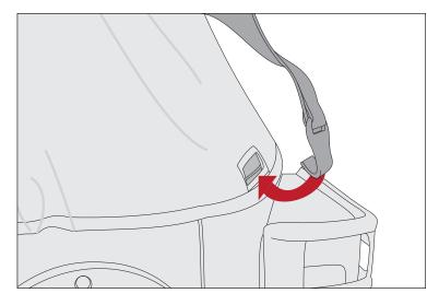
27. If desired, rear window can be rolled upwards, secured with two rear straps, and fastened to top with snaps located under top flap.
