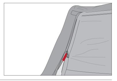
21. Loop top corner strap through plastic holder at rear corner of vehicle. Tighten strap and repeat for opposite side.
