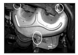
Step 9. Remove the passenger and driver side heat shield bolts. Remove both heat shields. Do not discard the passenger side, it will be reused later. A bolt penetrating spray may be needed.
