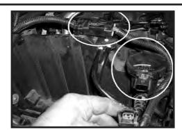
Step 4. Remove the EVAP solenoid connector and power junction connector. The red slide tab will have to be pulled out slightly to remove connectors. Remove the EVAP solenoid from the holder by sliding it up off of the tab and set aside. Remove the junction connector from the tray and set aside.
