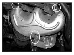
Step 13. Install the passenger side heat shield using the remaining two flange bolts and heat shield brace bolt.
