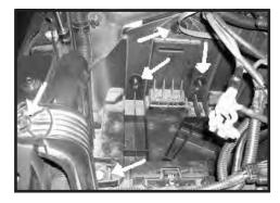
Step 3. Remove the three nuts and two bolts in the battery section of the tray.
