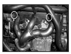
Step 12. Install the passenger side header, and gasket. Install the upper flange bolts with the exception of the top left and right bolts. These bolts will be used to hold the factory heat shield in place. Install the down pipe flange bolts on each side
