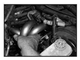
Step 11. Install the driver side header, and gasket.
