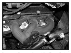
Step 10. Remove the two down pipe flange bolts on each manifold. Remove the remaining bolts holding on each manifold. Remove both manifolds and set aside. Remove any remains of the old gasket material that is left on the head. Be careful not to gouge the aluminum cylinder head.
