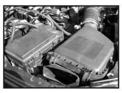
Step 16. Reinstall the battery tray, battery, power fuse box, steering reservoir and bracket, and air box. Start motor and check for exhaust leaks.
