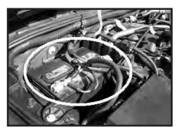
Step 1. Disconnect the battery terminals from the battery and move aside. Remove the battery hold down clamp. Remove the battery.
