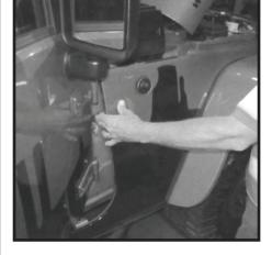
Tighten M6 x 20mm Flange Hex Head Bolt and M6 Flange Nuts before reinstalling fender on vehicle. When fender is being installed remember to connect antenna cable.
