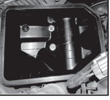
**51** - With Air Box in the correct location, 90deg Elbow attached to lower Air Box inlet and aligned with the Air Tube. Carefully remove Air Box and 90deg Elbow together. Mark the position of the 90deg Elbow to Air Box as shown. remove elbow for step (52).
