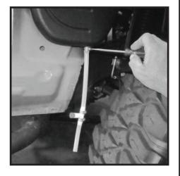
**87**- Adjust (4) air box sealing clamps full open. Clamps are designed to slip under lower air box flange and over flange and ribs of upper OE air box. Place clamps as shown (arrows). Secure but do not tighten clamps.
