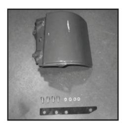
4 - Cowl should be aligned with outer edge of fender. Fender can be placed onto body to double check cowl placement (front to back). The left side fender can be used as a guide if needed.
