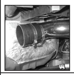
**73**- Inspect Cowl "Z"-Bracket to Main Body alignment. Adjust Main Body and Cowl "Z"-Bracket to align mounting holes. If needed Cowl "Z"-Bracket can be adjusted (bent) to align all holes. 71 - With sealant applied to main body outlet slip Hose Clamp onto Mian Body outlet. Position snorkel Main Body onto vehicle sliding outlet into Coupling as shown. Slide Hose Clamp over Coupling but Do Not tighten.
