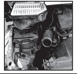
**45** - Inspect front of Ait Tube. Air Tube should rest between shock tower and power steering pulley. Confirm Air Tube does not make contact with any other component.
