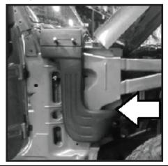
**75** - Check alignment of cowl cover and Main Body. Insert M6 x 20 Phillips head screws to align cover, Main Body and Cowl "Z" - Bracket.
