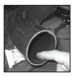
**55** - Apply a thin film of sealant around end of Air Tube. An excessive amount may cause the elbow to slide off air tube when tightened.
