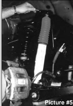
7. 2½" Lifts: Reattach track bar in original axle mount (it may be necessary to rotate steering wheel left or right to align bolt hole).
