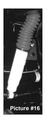
9. 2½" Lifts: Reattach sway bar links to axle housing and skip to step 10, unless purchased extended rear sway bar end links.
