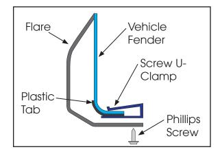
11. Use a 10 mm socket wrench to reinstall factory bolts. Complete rear flare installation.
