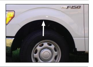
5. Install Front Flare Inner Piece using a supplied Phillips screw through installed Small Screw U-Clamp. Use factory screws and 7/32" socket to attach inner piece to factory holes.
