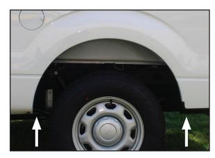
9. Hold flare to vehicle and using a marker or grease pencil mark locations of four holes in flare on sheet metal. Wrap a Plastic Square Tab around sheet metal over four marks. Install Long Screw U-Clamps over four Plastic Square Tabs.
