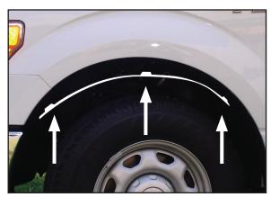
6. Hold flare to fender and install factory screw into factory hole toward rear of wheel well using 7/32" socket. Continue to hold flare and drill through bumper cover with a 1/4" drill bit using forward most hole in flare as a guide.
