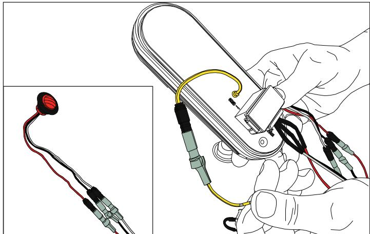
5. Connect the Wire Harness(#3) into the factory wire harness. Using the supplied No 8 Socket Head Screws(#9), attach the Flush Mount Light to the vehicle.
