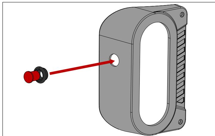
3. Affix the Oval Light Grommet(#5) into Tail Light Mount(#1&2). Press the Oval Light(#4) into the Oval Light Grommet(#5).
