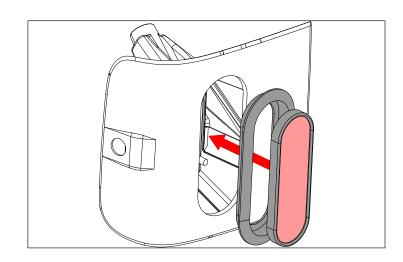
6. Affix the round light grommet(#7) into tail light mount. Press the round light(#6) into the round light grommet.
