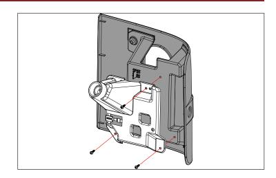
5. Affix the oval light grommet(#5) into tail light mount. Press the oval light(#4) into the oval light grommet.
