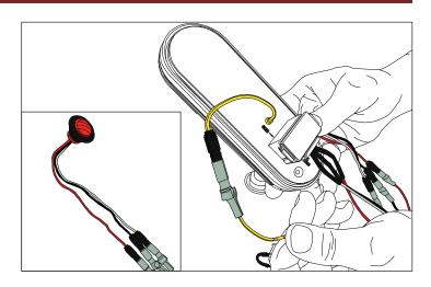
8. Connect wire harness into factory wire harness. Reusing the OE tail light mounting bolt, attach flush style light to vehicle.
