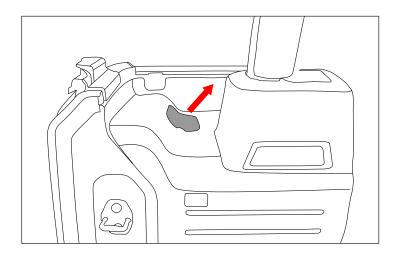
2. Using either a 10mm or T40 torx socket, unscrew OE mounting bolt and carefully pull tail light away from vehicle. Unplug tail light by sliding red tab first. Then press down on gray tab and gently pull plug from light.
