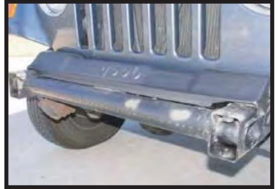
Step (2) Position the new front bumper up to the frame
