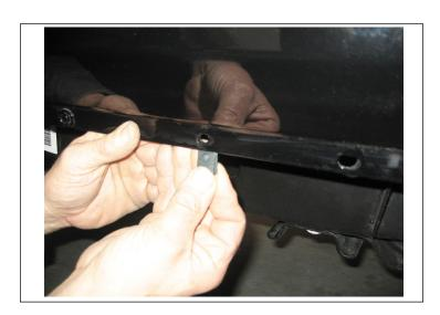
5. Place part on vehicle, making sure to line up edges of part with edges of vehicle. Ensure that all tape tabs are accessible.
