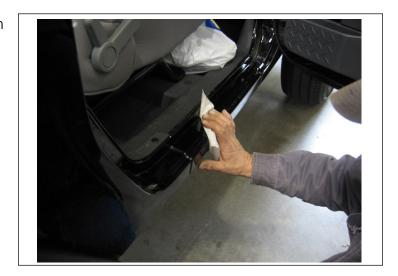
3. Locate the four factory holes in the rocker.
