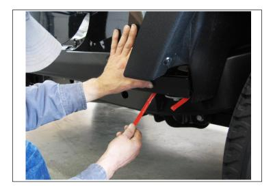
11. Toward the front of the vehicle, pull 1/2" tape liner tab 5. Press firmly on the part following tape liner removal.
