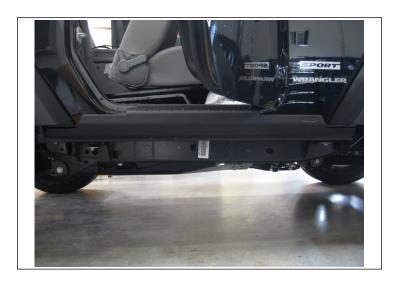
14. Using a #2 Phillips screwdriver, start a screw through each hole in side panel and through clips installed in step 4. Once all screws are started, tighten.
