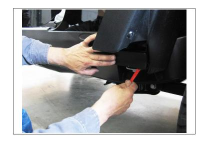
12. Toward the rear of the vehicle, pull 1/2" tape liner tab 6. Press firmly on the part following tape liner removal.
