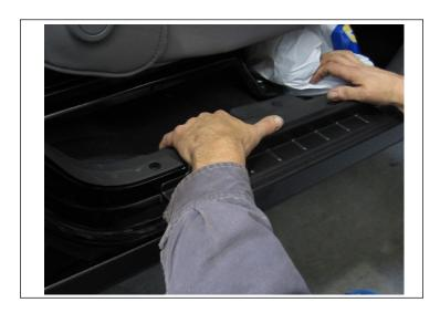
9. Toward the rear of the vehicle, pull 1/2" tape liner tab 3. Press firmly on the part following tape liner removal.
