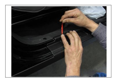
8. Press down firmly on part along the length of the sill.
