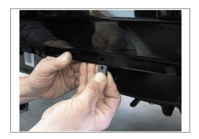
6. Place part on vehicle, making sure to line up edges of part with edges of vehicle and holes in part with clips installed in step 4. Ensure that all tape tabs are accessible.
