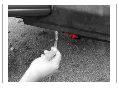
11. Once all tape liners are peeled, press down on entire length of part applying strong force to taped areas.
