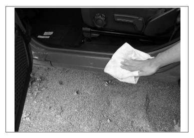
3. Place part on vehicle, making sure to line up edges of part with edges of vehicle. Ensure that all tape tabs are accessible. Firmly press on exposed areas of tape to tack Trail Armor in place.
