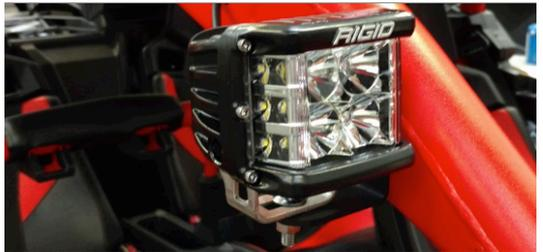
**Wiring: Wire your lights according to the instructions included with the light. Take care to avoid any heat sources and sharp or abrasive surfaces.**
