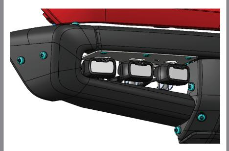
**STEP: 3** Use the supplied wiring harness to supply a power source to the lights.
