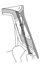
Install the tension strap through the loop on the strap sewn into the top. Pull tight and secure with hook and loop.
