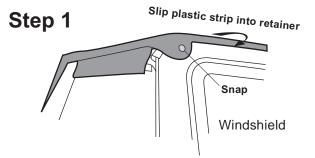
Lay the top out on the vehicle and insert the plastic strip into the channel over the front windshield. Now snap the front two snaps. Open the hook and loop flap on the sides over the front doors
